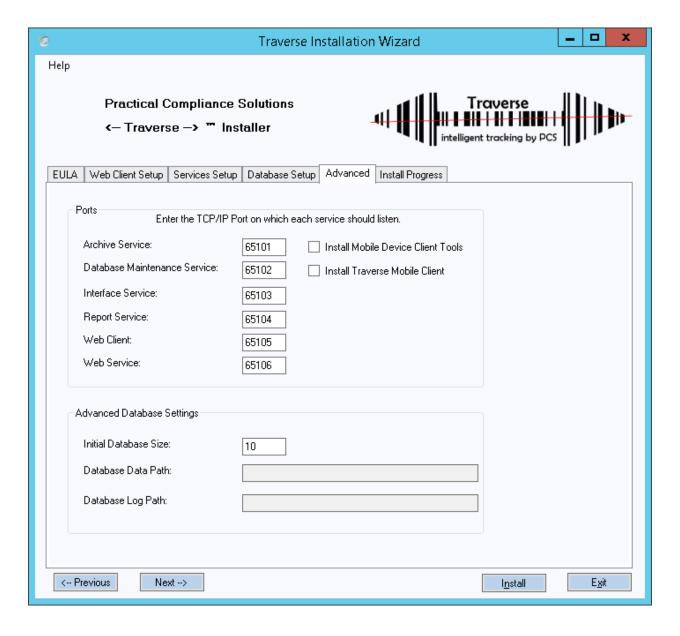
You can enter an initial database size and or installation path for the database files. When creating a new database on SQL server, the minimum size of a new database must be greater than or equal to the size of the SQL Server system database named model. By default the model database is 2MB for SQL 2008 and 4MB for SQL 2012. The default size for Traverse is 10MB.
