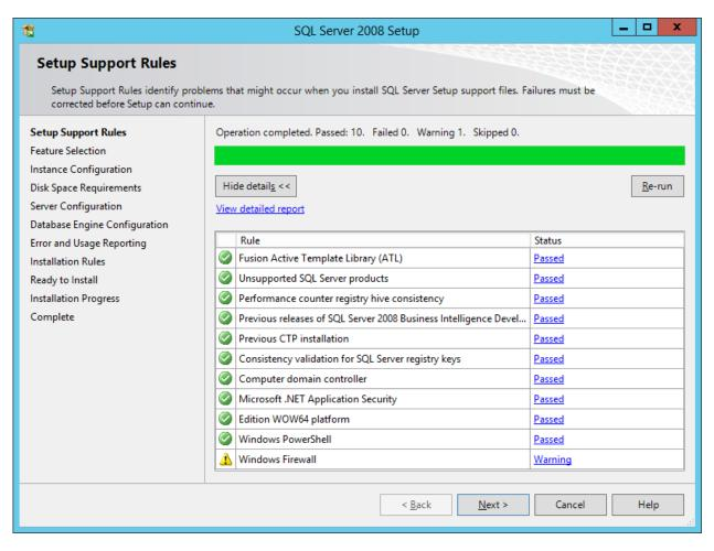
The Traverse installer will adjust the Windows Firewall allowing TCP Port 1433 and UDP 1434 for pass-through.
