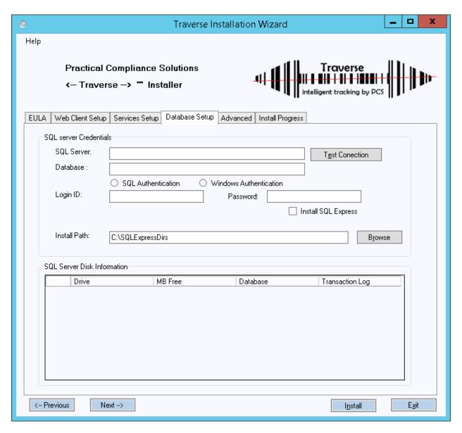
Enter the SQL Server credentials and click the "Test Connection" button. Upon successful connection to SQL Server the disk and available drive space will appear. Select the disk where the Traverse database and transaction log should reside.
