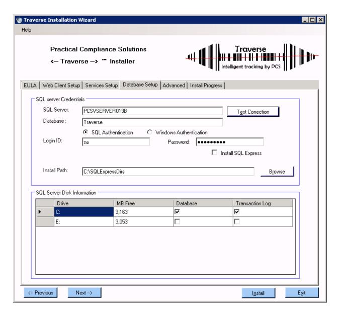
If you are installing a version of Traverse that is packaged with SQL Express, you will see the screen below. By checking the Check Box labeled "Install SQL Express, the Traverse installation package will install SQL Express." Refer to the "Installing Traverse with SQL Express" section of this document for more information.
